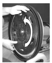
3. Mount the sanding disc. NOTE! Mount counterclockwise!
