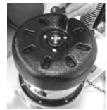
2. Loosen the screws on the motor cover.
