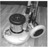
3. b) Raise the handle to an upright position, pull out the front carry handle.
