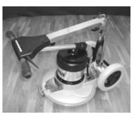
3. a) Raise the handle to an upright position, pull out the front carry handle and fold the handle shaft.
