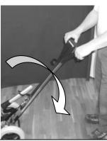
Lower the handle shaft to the desired position. The machine will not start if the shaft is not lowered at least 10°..
