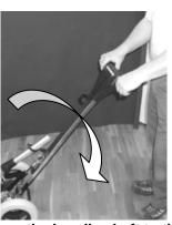
2. Lower the handle shaft to the desired position. The lower position with relaxed arms, the easier the machine will be to handle. Release the button.
