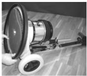
1. Tip the machine backwards and remove the dust skirt.
