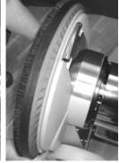
Place the dust skirt in the intended notch on the rubber strip.
